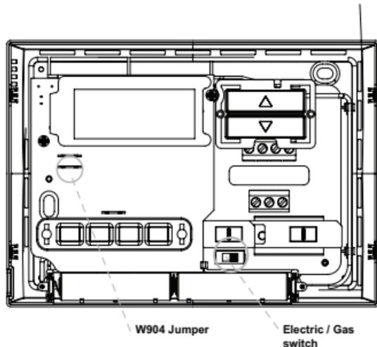
If you have either a gas or oil furnace, set the switch to GAS.
