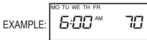
This display window shows that for the 1st weekday period, the start time is 6:00 AM, and 70° is the programmed temperature (this example reflects factory pre-programming).
